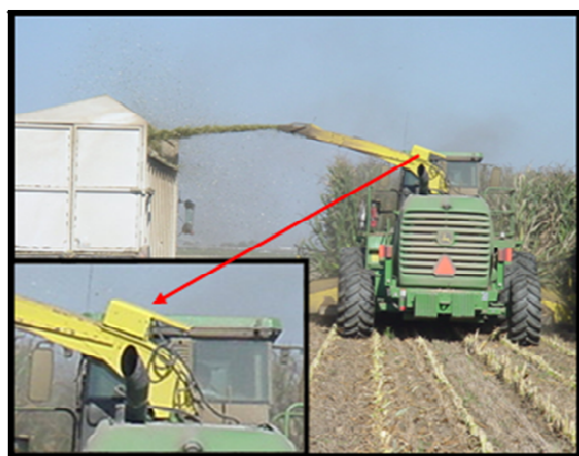
Figure 8: Prototype NIRS sensor mounted on forage harvester spout.
