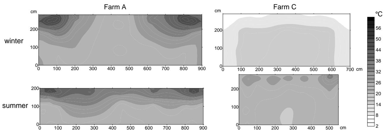
Figure 2. Contour map of temperatures recorded at 20-cm depths of the silo face in two farms of group A and C during winter and summer (Tabacco and Borreani, 2002).
